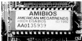
Fig. 1. Block BIOS, or ROM BIOS (stands for basic input/output system), is an example of firmware (middleware). The PC uses BIOS to start up the operating system
