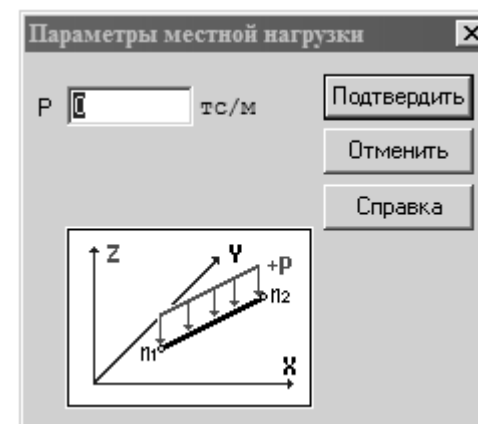
Fig. 1.64. The applying of the loading in regular intervals distributed on length of a rod.
