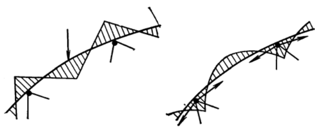
Fig. 17.11. Bending moment diagrams for the top chord of a bowstring truss
