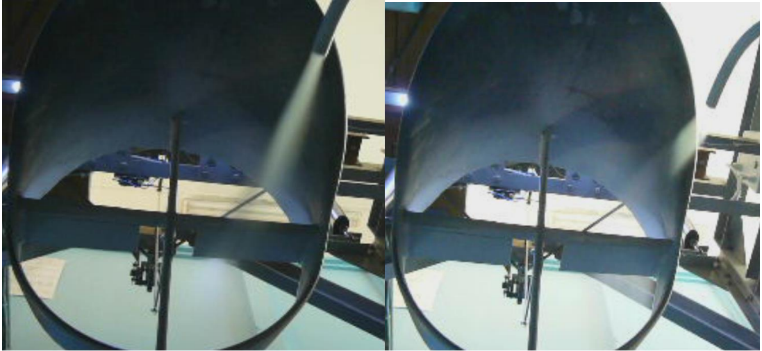
Figure 8 - CPW model in wind tunnel T-5, airflow V=35 m/sek. Smoke visualization
