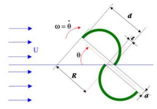
Scheme of a Savonius rotor: U is the wind speed;  $\theta$  is the angular azimuth for a blade;  $\omega$  is the angular speed; R is the rotor radius; d is the blade chord; a is the gap; e is the overlap
