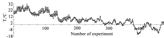
Fig. 2. Measured values of air temperature during experimental period
