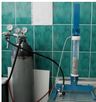
Fot. 1. Stand for testing mud and cement slurry leakages into layer.
