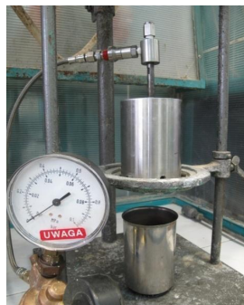
Fot. 2. Stand for testing cement slurry leakages into slit.
