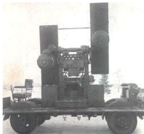
Figure 9. The radio-searcher B-3: the device for determining the elevation angle.
