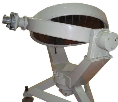
Fig. 1. Three axis test table for INS dynamic testing.
