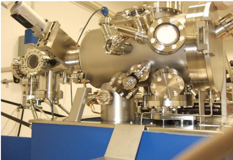
Fig. 6.16. Photo of the ALD plant
