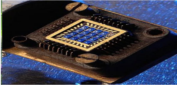
Fig. A3.3. The chip with the spin transistors
