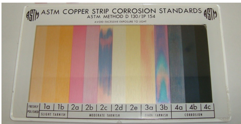
Fig. 8. The standard samples for determination copper strip corrosion
