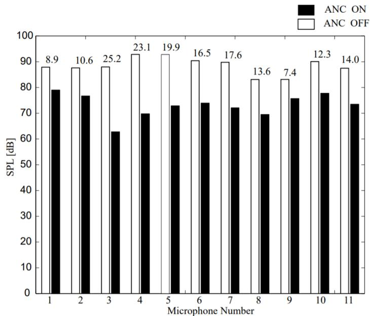
Table 2.4-Performance of the ANC system due to simulated propeller noise, 2×BPF, 910 rpm (121 Hz)
