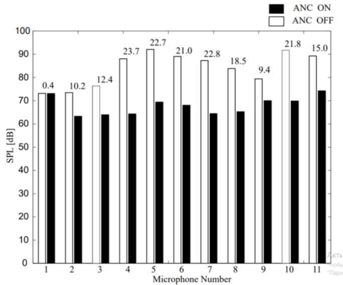
Table 2.3- Interior sound attenuation at 61 Hz, acoustic sensing
