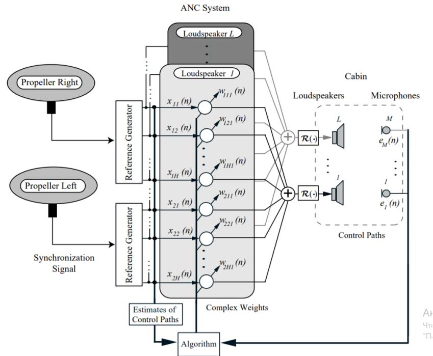
Fig. 2.3-The control system for active control of periodic noise.
