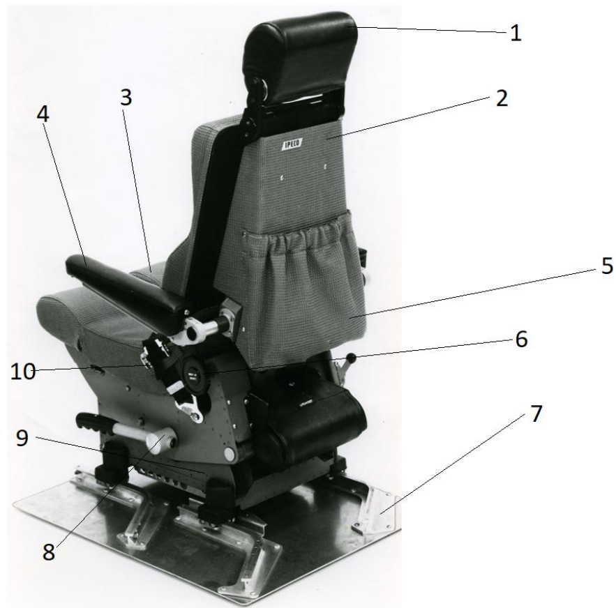
Figure 2.6 - Pilot's seat real view: 1 – headrest, 2 – seatback, 3 – seat bottom, 4 – armrest, 5 – pocket, 6 – seat base, 7 – rails, 8 – recline adjustment control, 9 – lumbar adjustment handwheel, 10 – straps.
