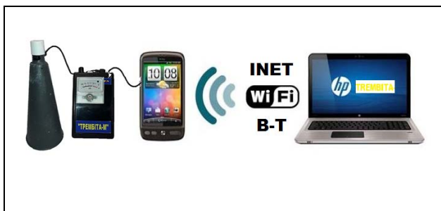
Fig. 1. The appearance of the acoustic receiver unit and block diagram of the operation of the module "Trembita-Corona M"
