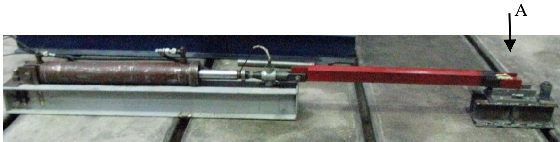
Figure 4.19 - General view of the XZ latch test stand
