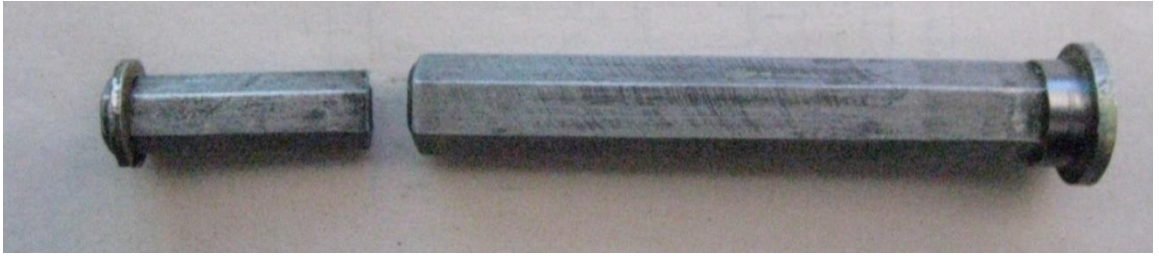
Figure 4.21 - General view of the axis destroyed during static tests of the XZ latch
