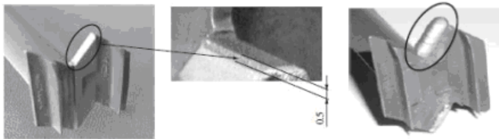
Figure 1.5 – Low pressure turbine shroud: welding and MSC coating
