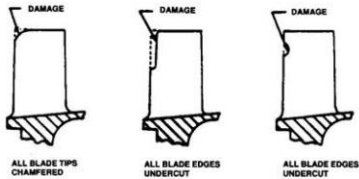
Figure 1.3 – Types of blade damage
