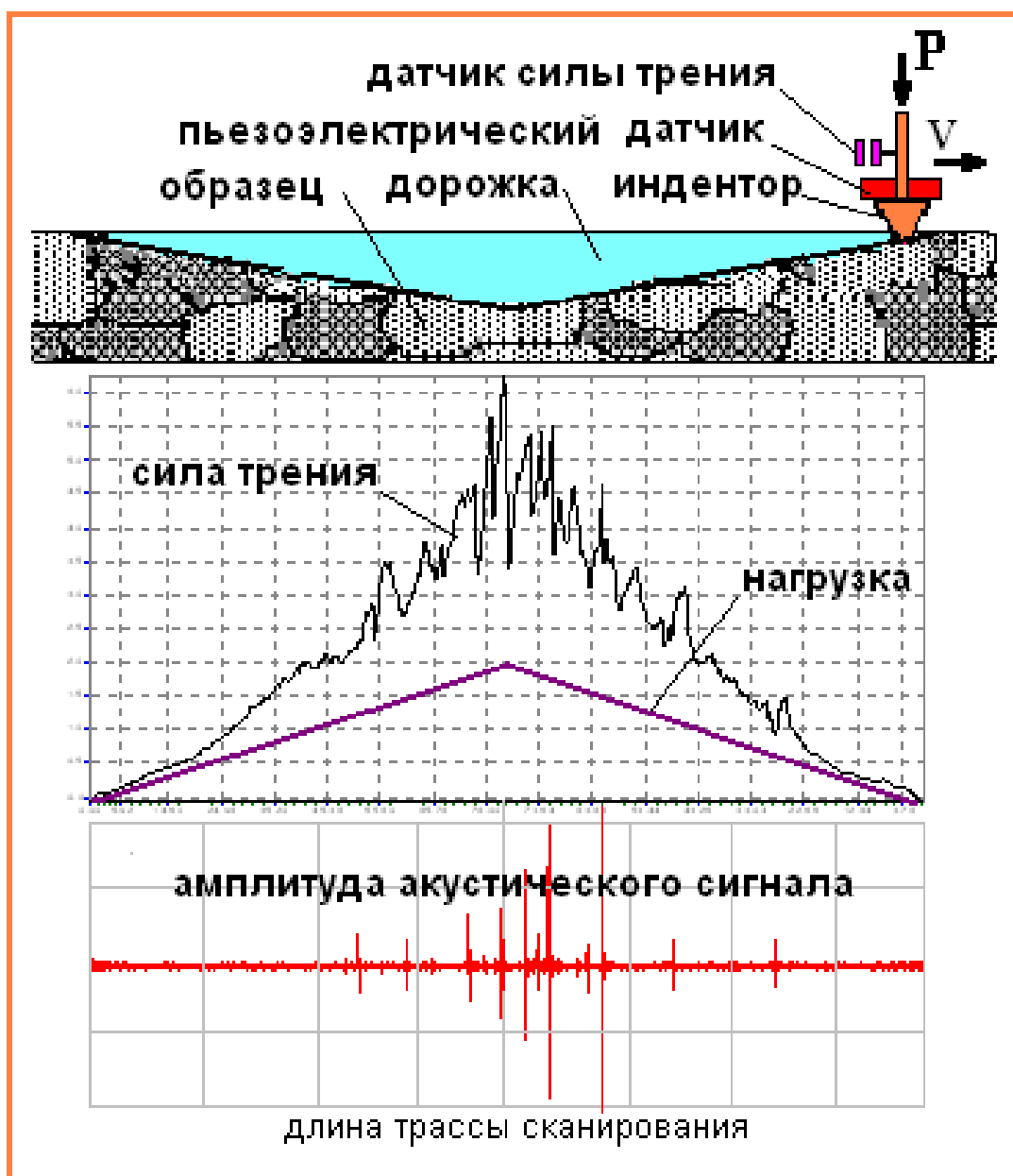
Figure 3.1 – Scheme of scratch testing of coating adhesion
