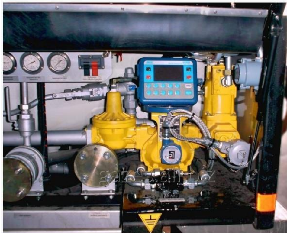
Figure 3.2 – Mechanical gas meter type MA-7
