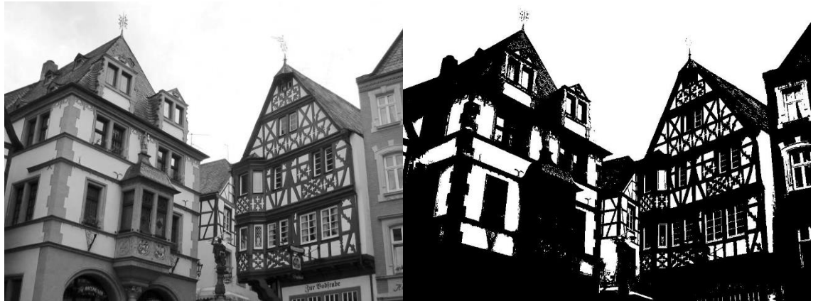
Fig. 3.8. Original image and after binarization with Otsu threshold
