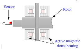
When calculating for the AMB several factors should be considered: the air gap is needed in order to prevent collision with casing; the rotational speed needs to be calculated in order to calibrate the sensor signal; the electro-magnetic force depends on the loop count, the current, the wire size, and the presence of an iron core.
