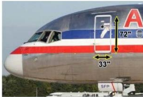
Figure 2.2 - Commercial standards of main door sizing
