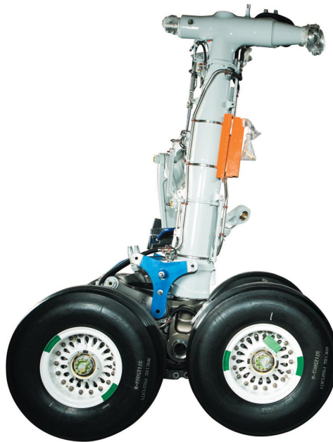
Figure 2.3. The white oleo-pneumatic shock strut cylinder is clearly visible in this image of part of one of two main landing gear legs for the Boeing 787.
