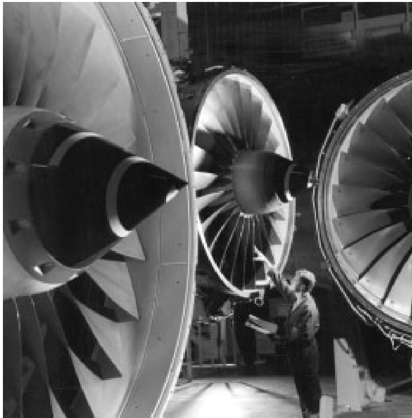
Fig. 1.8 – Fans of commercial Rolls-Royce Trent engines made of Ti-6Al-4V
