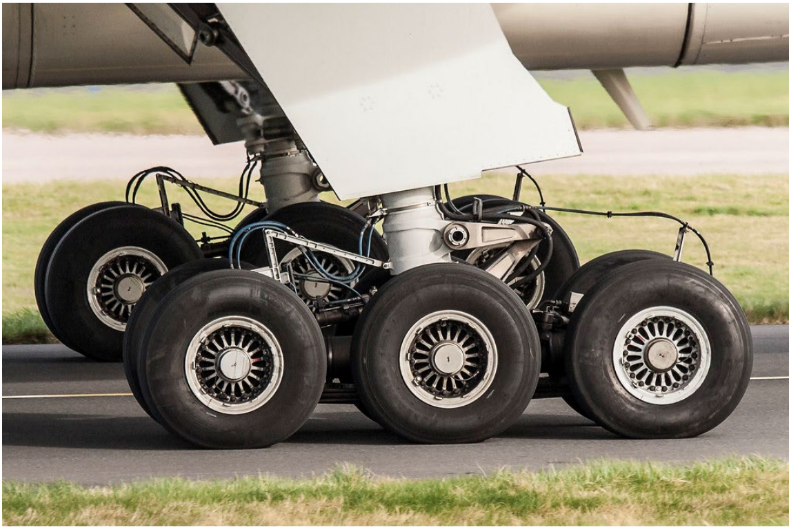
Fig. 1.4 – The main landing gear of Boeing 777 primarily uses forged parts of Ti-10V-2Fe-3Al
