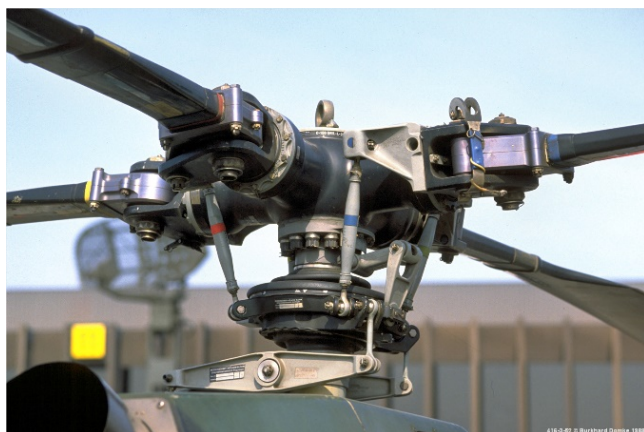
Fig. 1.15 – Forged rotor head of the BO 105 and BK117 helicopters
