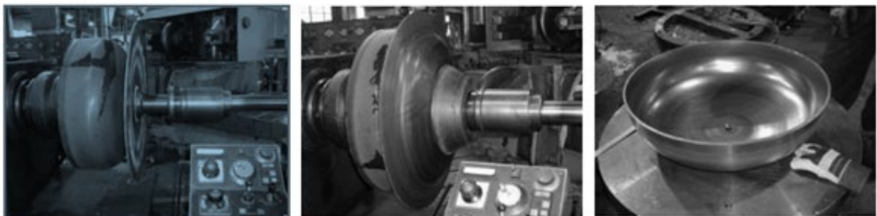
Fig. 1.18 – Sequences during spin forming of Ti-15-3 half shells
