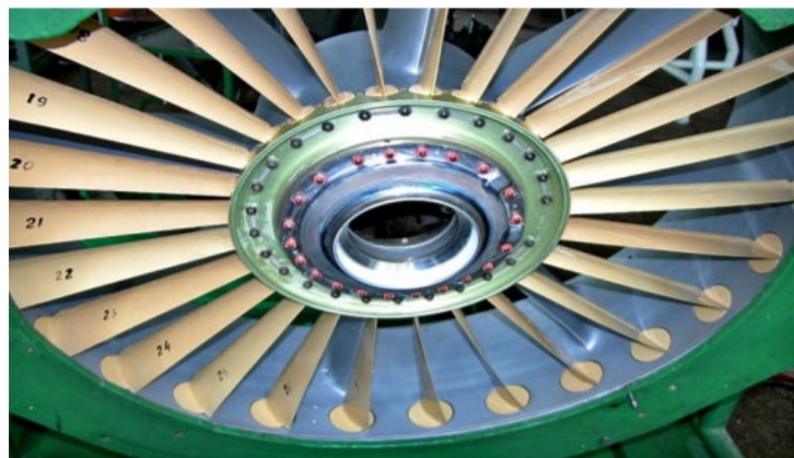
Fig. 2.6 – Inlet guide vanes with protective epoxy-polyamide enamel
