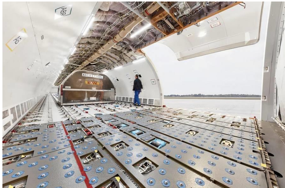
Figure 2.5. Main deck cargo compartment of the A330 after conversion
