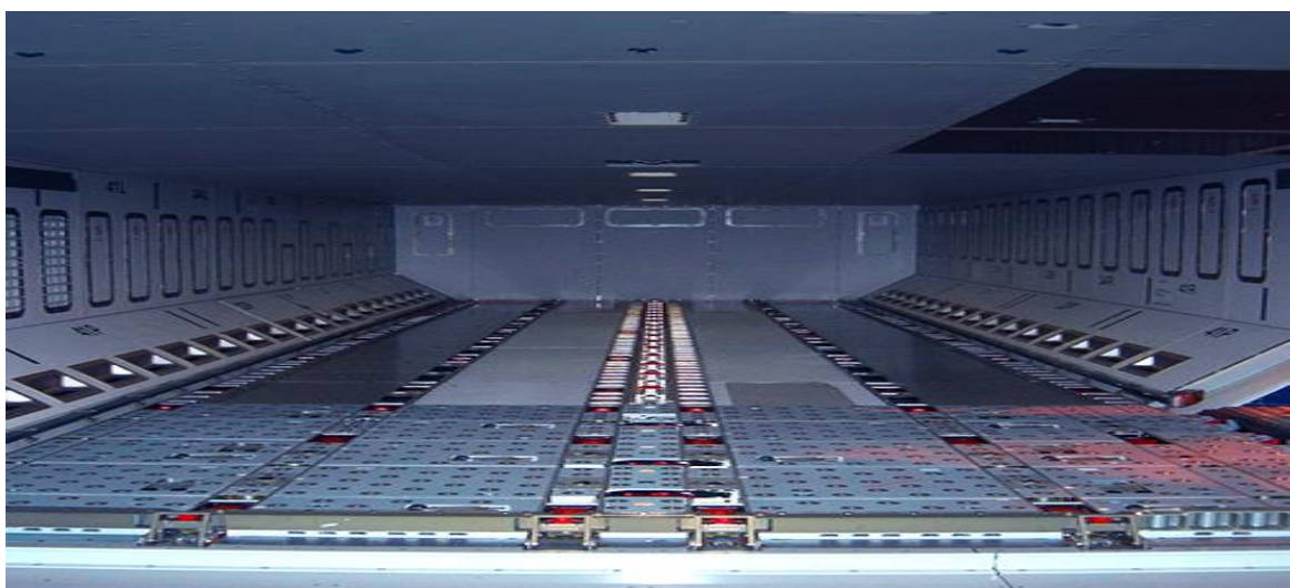
Fig.2.3 – A330 Lower Deck Cargo Loading System
