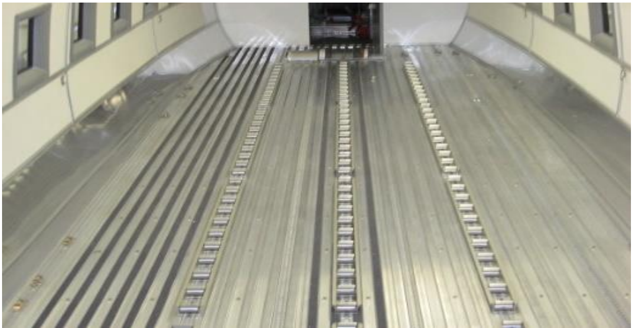
Fig.2.2 – Douglas DC-3 BT-67 roller floor: a – Aircraft; b – Sketch of the flooring system; c – fragment of the Roller Module System
