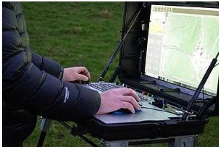
Fig. 1.1. An example of a portable ground control station of the UAV
