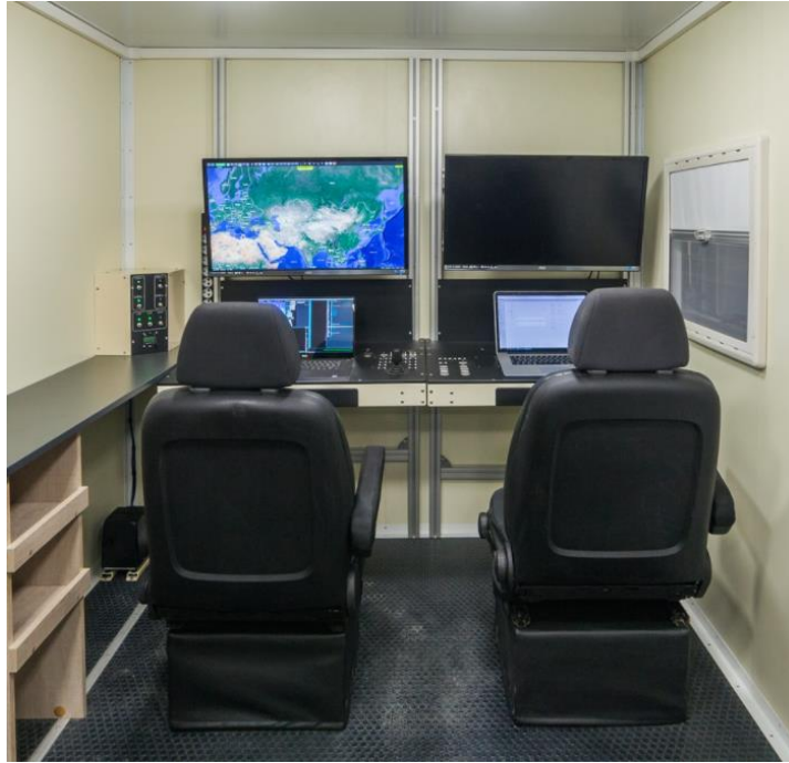
Fig. 1.2. An example of a full-fledged UAV ground control station
