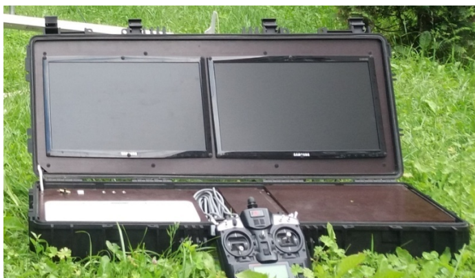
Fig. 4.11. General view of the ground control station (ground secured computer in a case)
