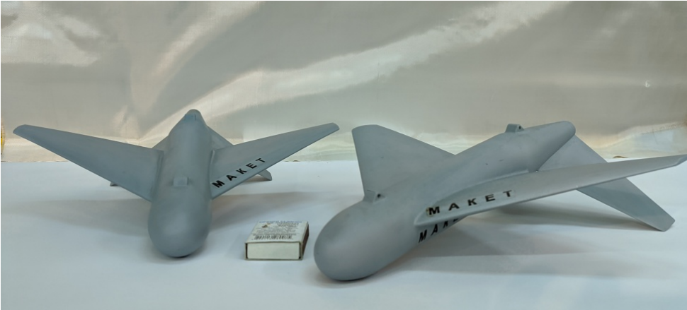
Fig. 4.28. General view planning self-guided mini-munition PMB-03 (mockup)
