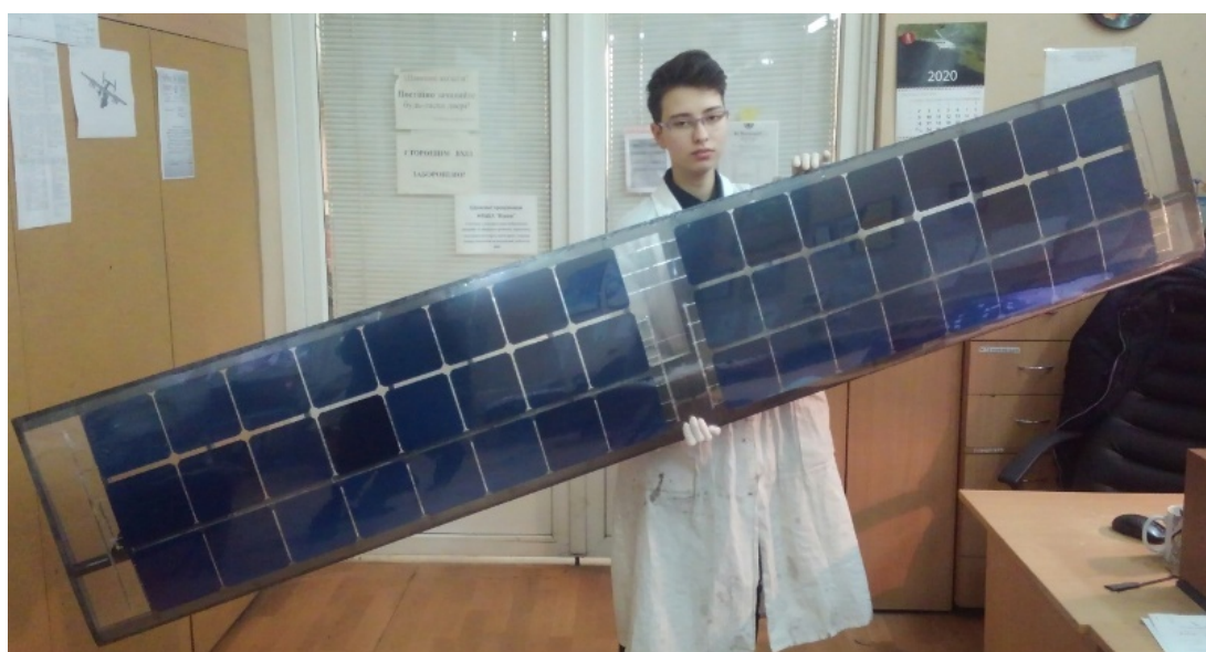
Fig. 6.18. Arrangement of the section of 48 solar cells on the horizontal plumage PS-11 «Krokus»
