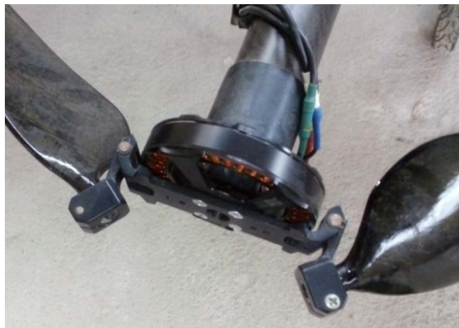
Fig. 2.61. An image of the propeller and the turning mechanism of the propeller blades in the «blades half-folded along the flow» position
