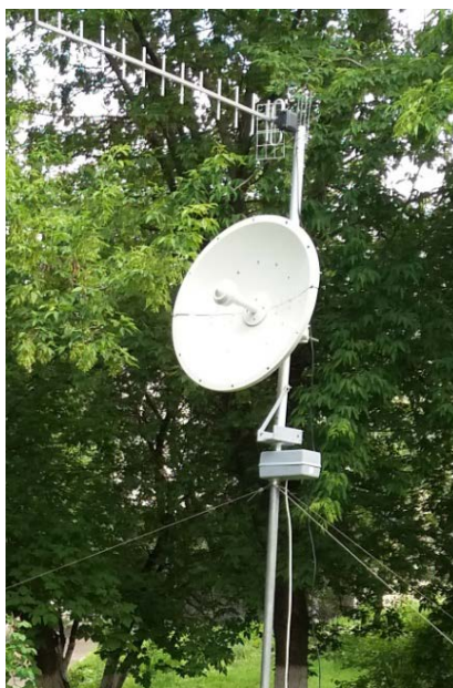
Fig. 4.12. Telescopic mast and automatic antenna deployment device in the direction of the UAV
