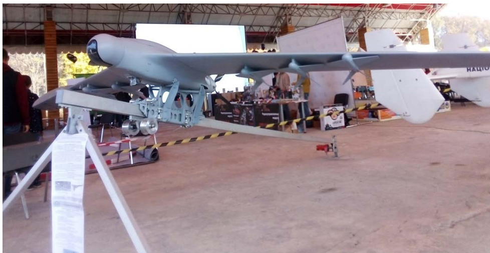
Fig. 4.30. Installation of a planning self-guided mini-munition onboard the aircraft unmanned carrier M-56 «Modul»
