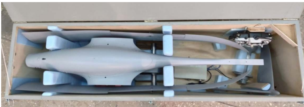
Fig. 4.8. General appearance and dimensions of the transport container for UAV «OVOD» M106 (container size 380 \text{ mm} \times 800 \text{ mm} \times 1400 \text{ mm} ; weight – 35 kg)
