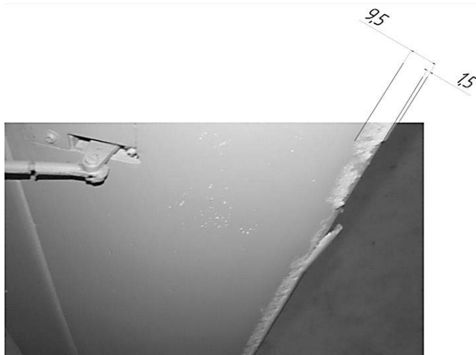
Fig. 2.14. Icing of wing leading edge (bottom view)
