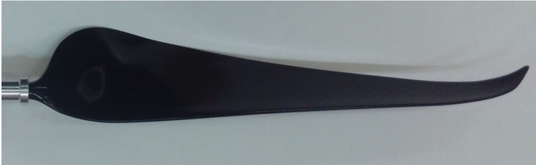
Fig. 2.65. Image of the blade of the proposed technical solution of the propeller
