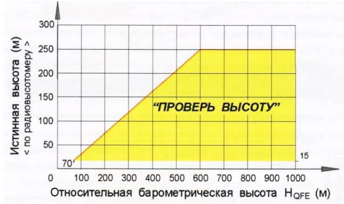
Figure 1.9. Mode 6 "Exceeding the threshold value of the difference between the geometric and relative barometric height".
