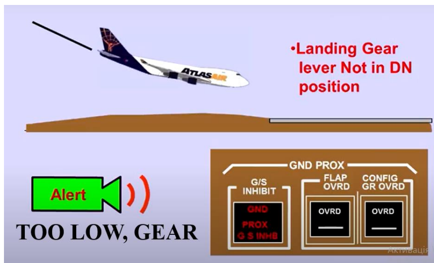
Fig. 2.6 System panel in mode 4 b)
