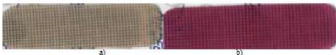
Fig. 3. Gaskets materials sampling: a – HI-TAK Tape TufSeal™ (HT3000); b – HI-TAK Tape (HT3935-7).
