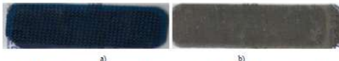
Fig. 2. Gaskets materials sampling: a – HI-TAK Polyurethane Conductive Gasket standard antenna gasket material; b – HI-TAK Polyurethane Fuel Resistant Conductive Gasket (FG 323000-XX).
