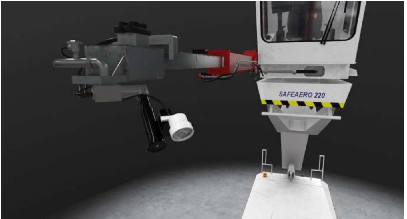
Fig.1.2.6 Spray unit of the Safeaero special vehicle
