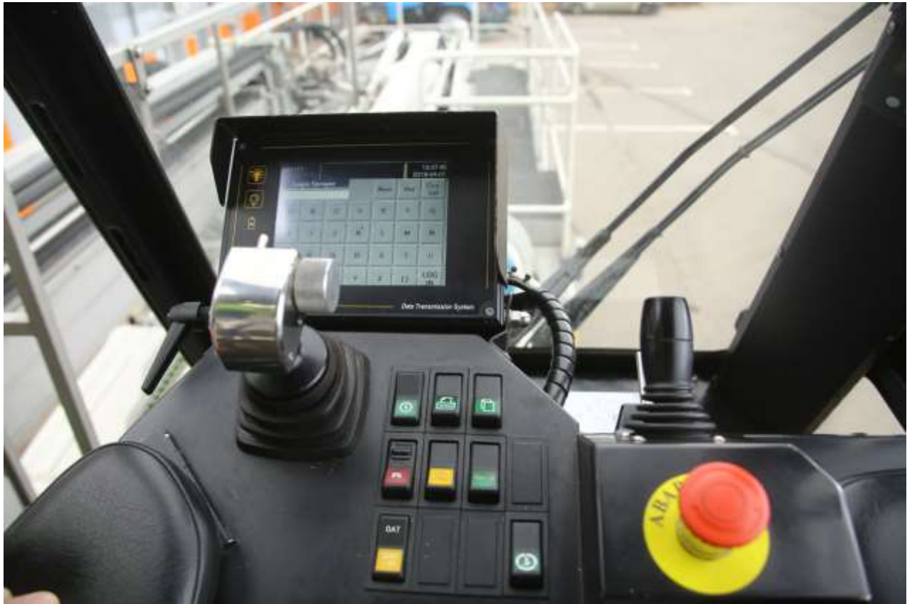
Fig.1.2.5 Boom and telescope control panel for special vehicles [9]: telescope control toggle switch; boom control toggle switch; joystick control telescope; switch of working liquid supply; lever control unit for spray heads.
