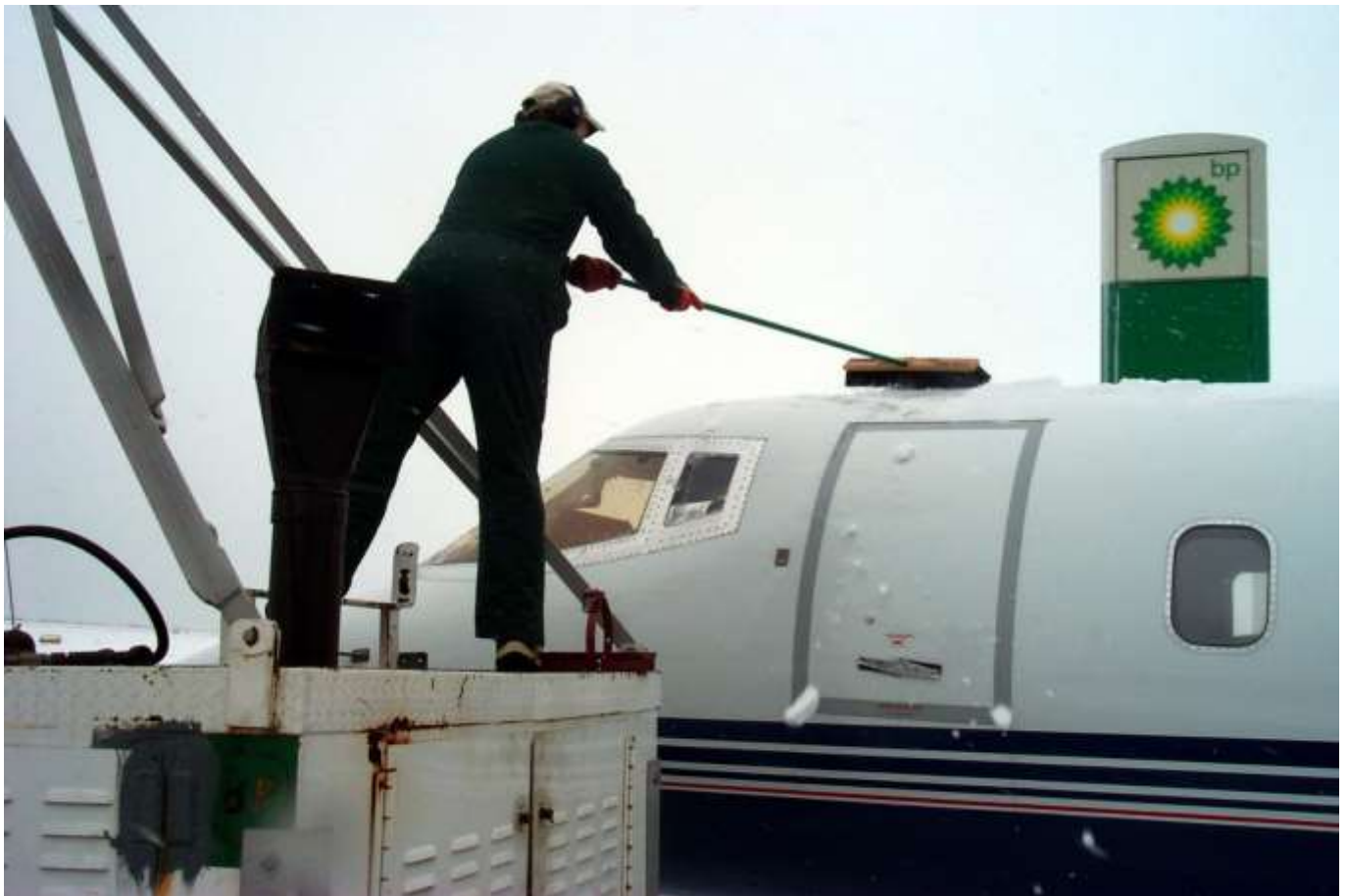
Fig.2.2.1 Mechanical de-icing the surface of an aircraft with a broom [22]
