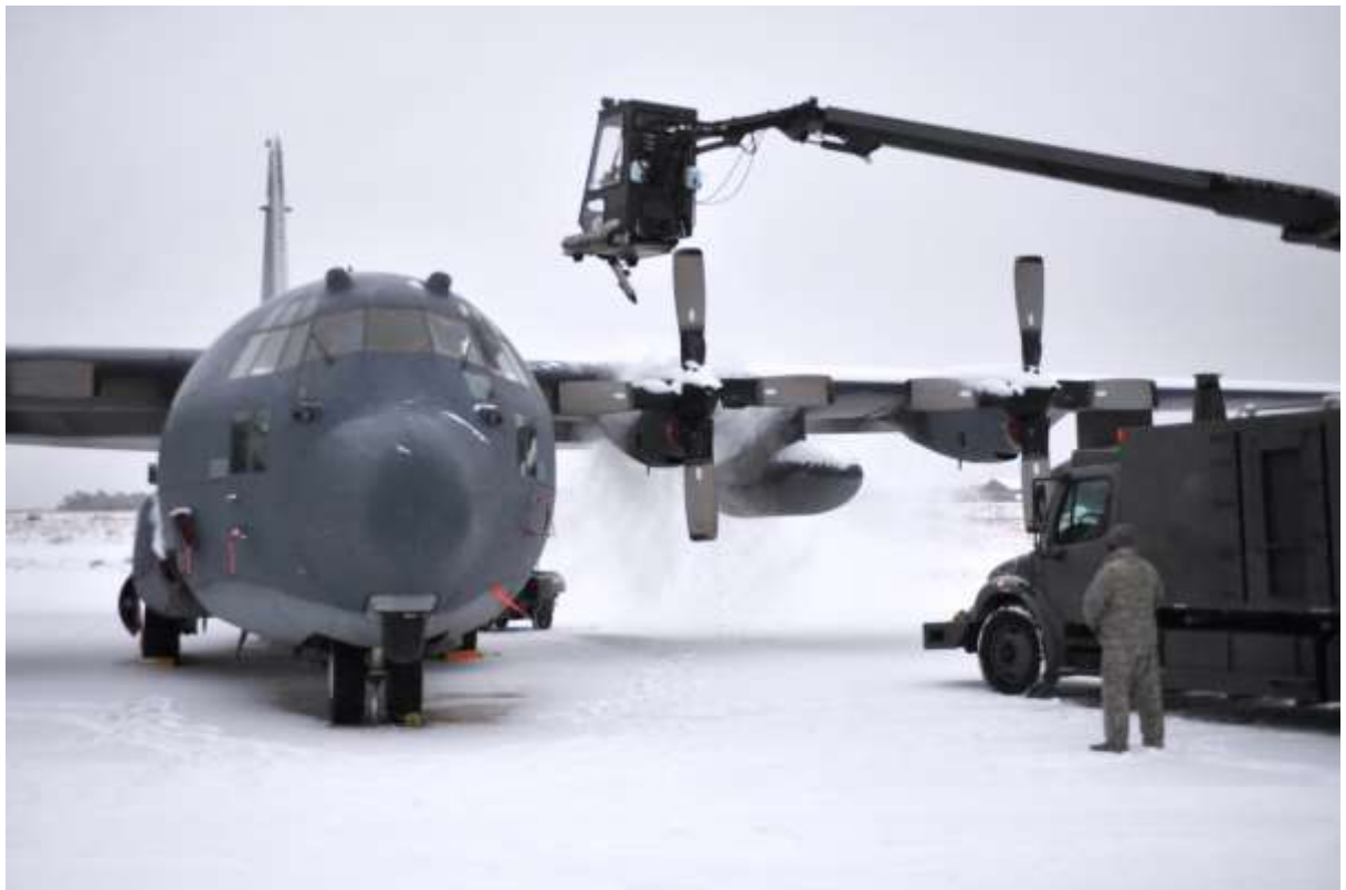
Fig.2.2.2.1 De-icing of aircraft by hot air flow [23]
