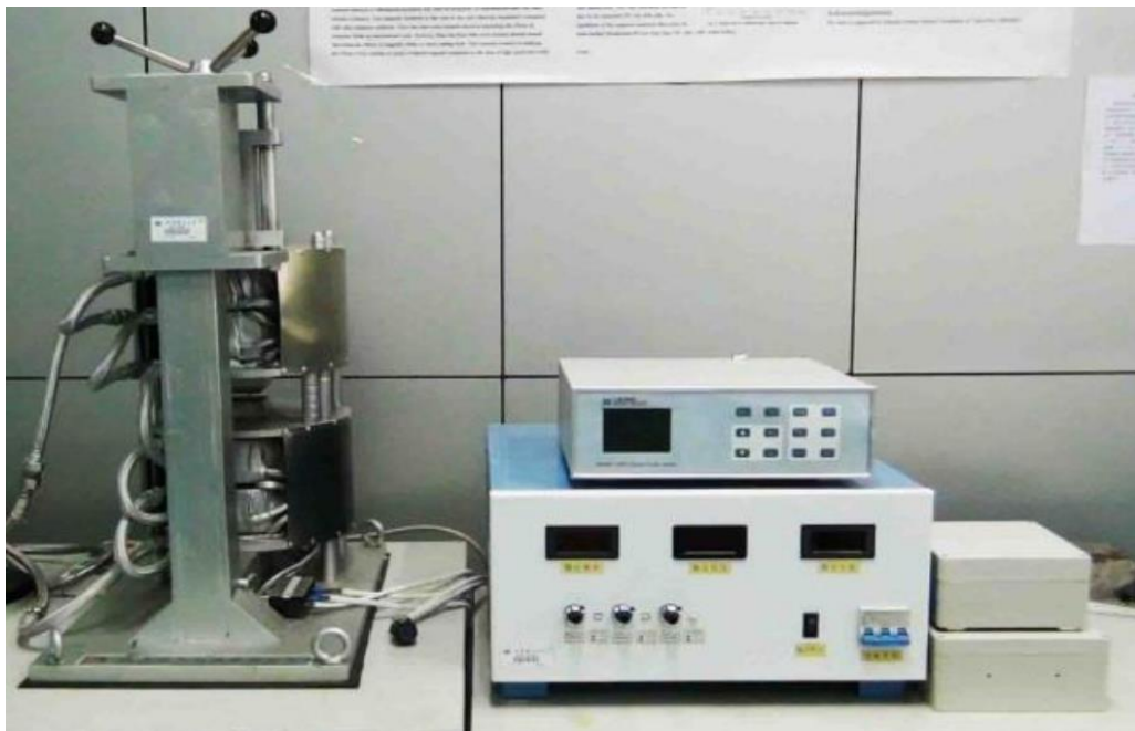
Figure 4.1 - Pulse magnetic field enhancement processing platform
