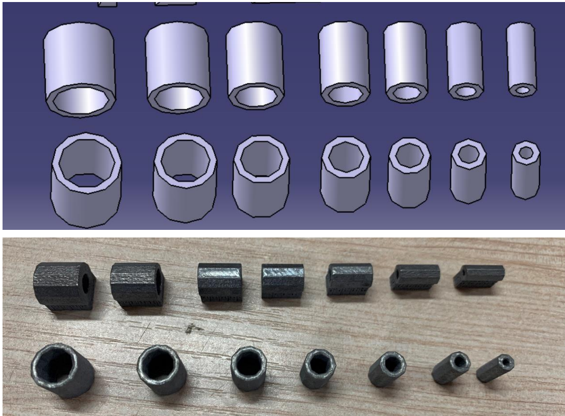
Fig. 3.22. Schematic diagram and renderings of forming rings of different radius.
