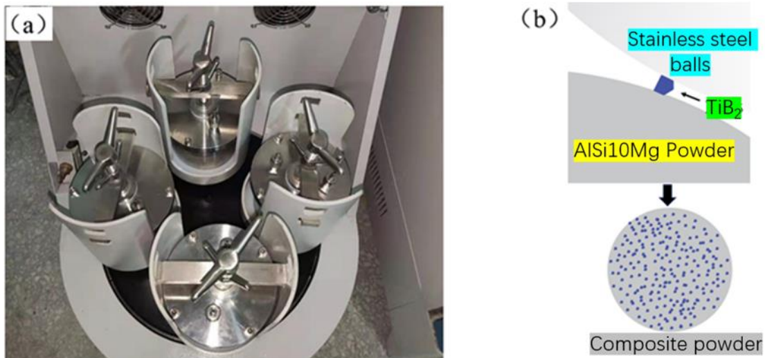
Figure 2.4. Low-energy ball mill: (a) low-energy ball milling equipment; (b) Schematic diagram.
