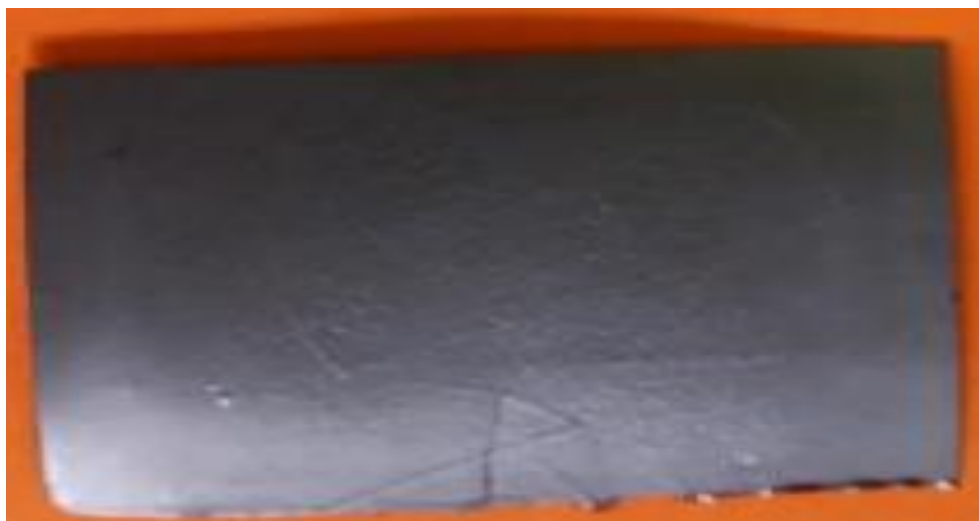
Figure 3.5 – Graphite film heater.
