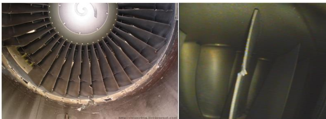
Рис. 3.8 Nicks, tears, dents in the fan and compressor blades of the engine CFM56-5B
