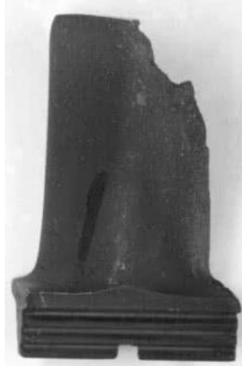
Рис. 3.5 Breakage of a part of the rotor blade of the second stage of the turbine of the Д-30КР-2 engine
