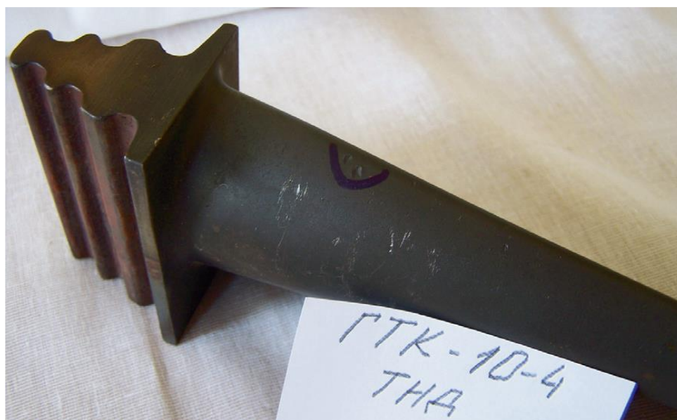
Рис. 3.4. LPG blade for gas turbine engine type GTK 10-4 with a nick..
