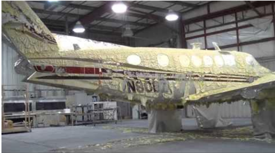
Figure 35– An example of stripping process
