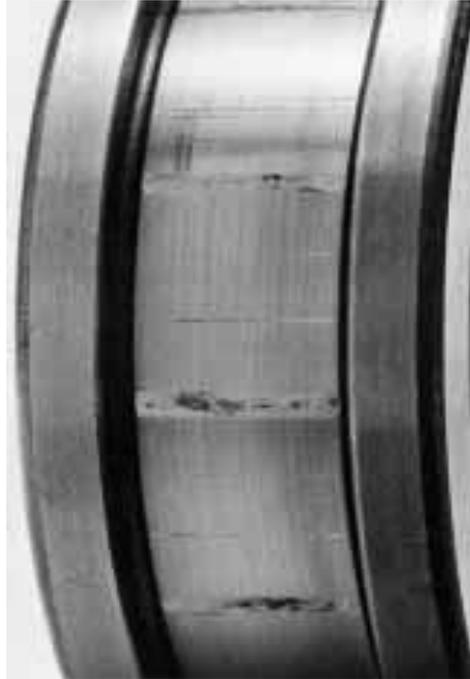
Figure 1.7 – Vibration damage to the ring of cylinder roller bearing.
