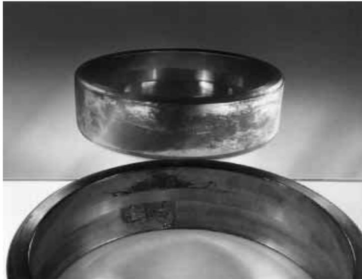
Figure 1.19 – Flaking in the raceways of the outer ring of a spherical roller bearing
