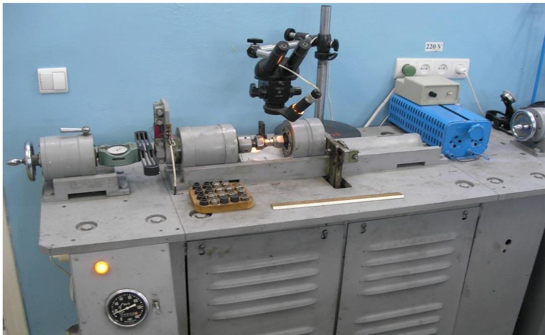
Figure - 3.1 Outward of settings MΦK-1 testing at fretting corrosion
