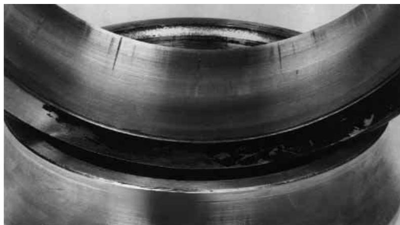
Figure 1.12 – Outer ring raceway of a spherical roller bearing with smear streaks caused by a blow against the inner ring
