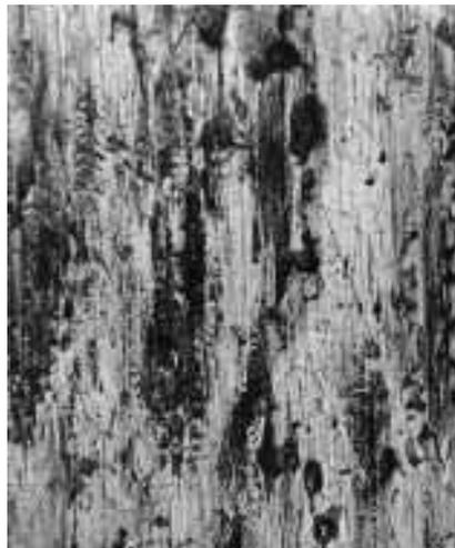
Figure 1.10 – Smearing on the surface of a roller from a spherical roller bearing – 100 × magnification
