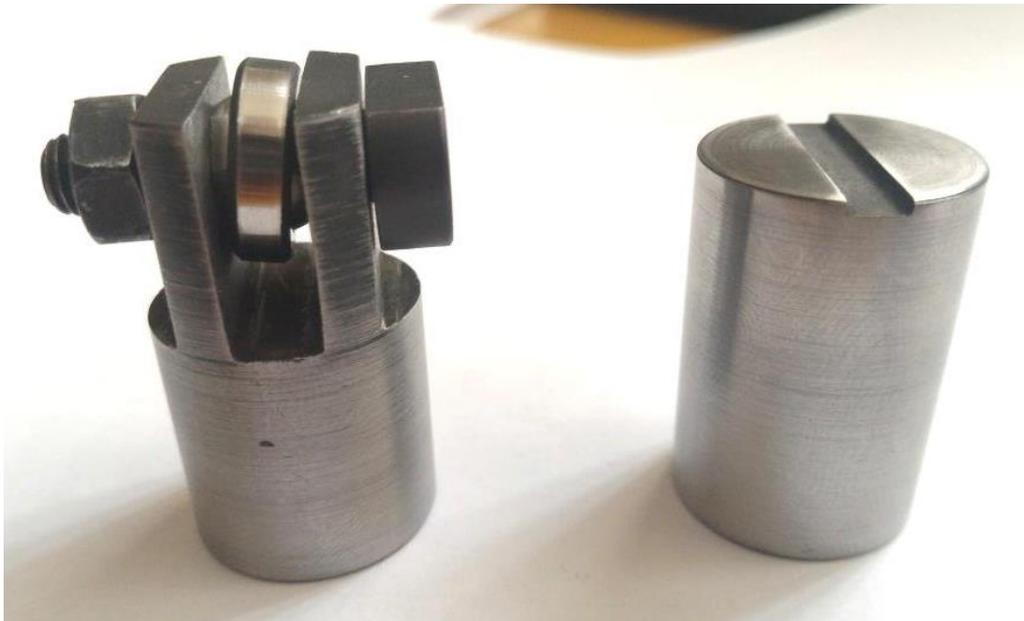
Figure - 3.5 Clips to hold the spherical plain bearings
