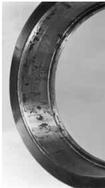
Figure 1.15 – Deep seated rust in the outer ring of a cylindrical roller bearing
