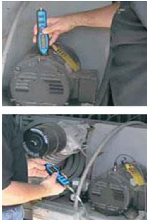
Figure 1.22 – Bearing vibration measurement
