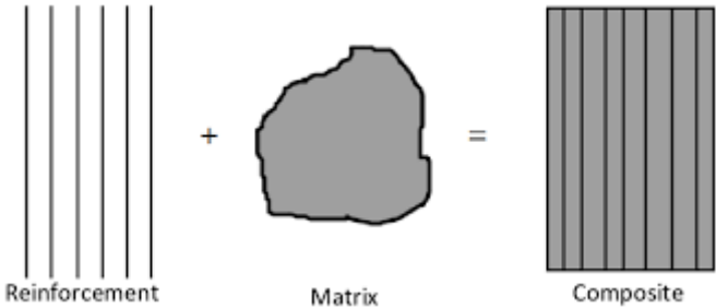
Fig. 1.1. Formation of composite material.
