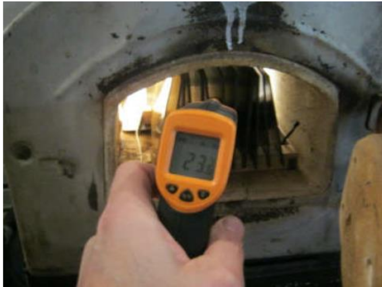
Fig. 2.20. Temperature control using infrared thermometer.
