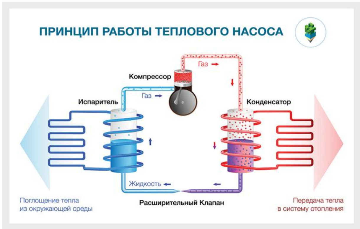
Figure 8 Operating principle of a heat pump
