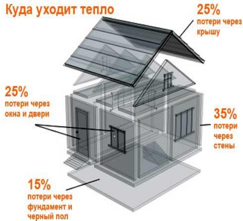
Figure 2 Percentage ratio of heat losses in a building
