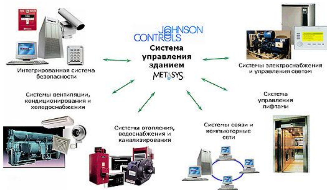
Figure 22 Building Control System: Johnson Controls Metasys
