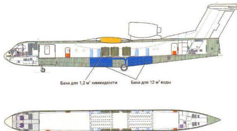
Fig. 1.3 Location of tanks
