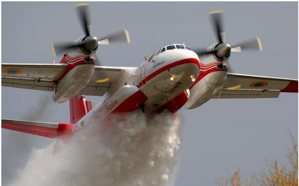
Fig. 1.1 An-32P in case of fire extinguishing.
