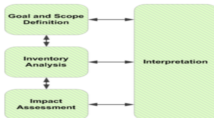
Fig. 6.1: Illustration of the general stages of life cycle assessment as described in ISO 14040
