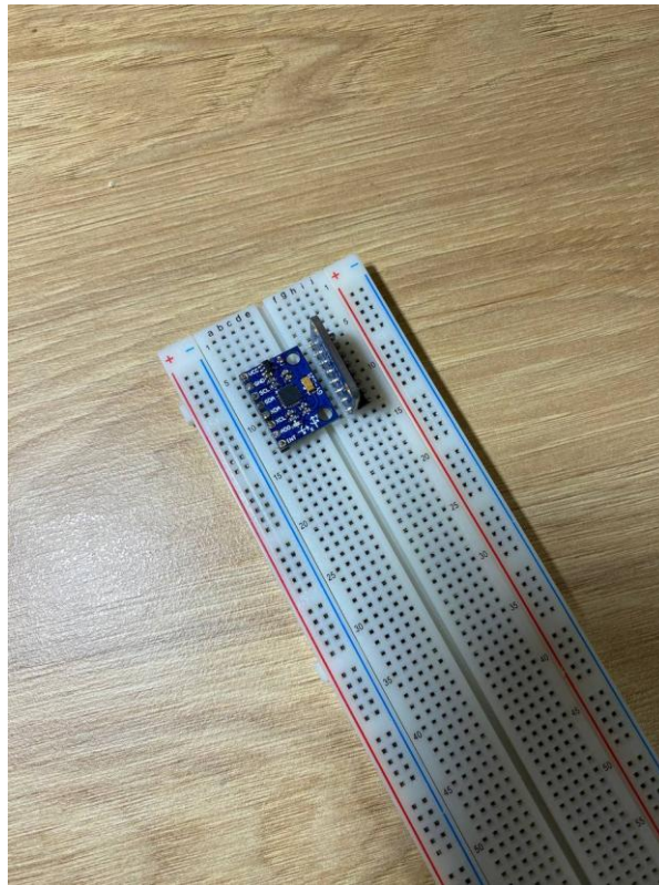
Fig. 4.8. GY-BMI160 connected to the Breadboard
