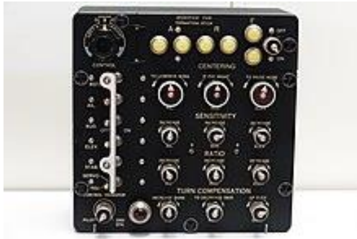
Figure 1.2. A World War II-era Honeywell C-1 autopilot control panel
