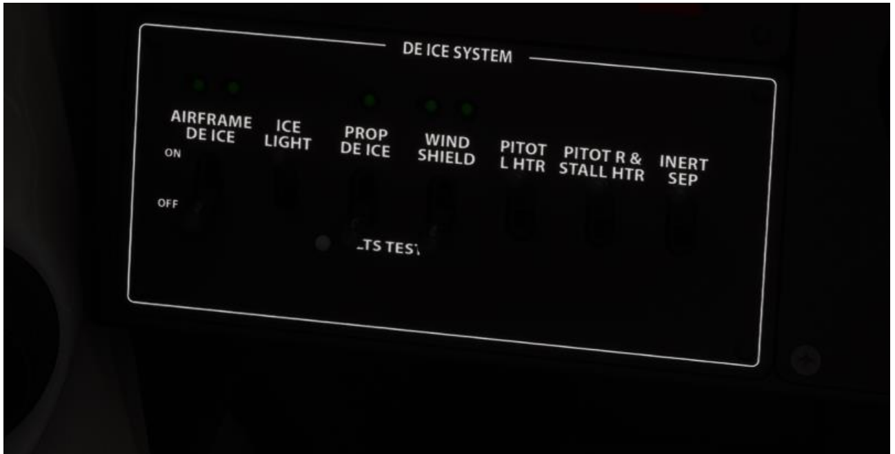
Figure 3.6. De ice system in TBM 930
