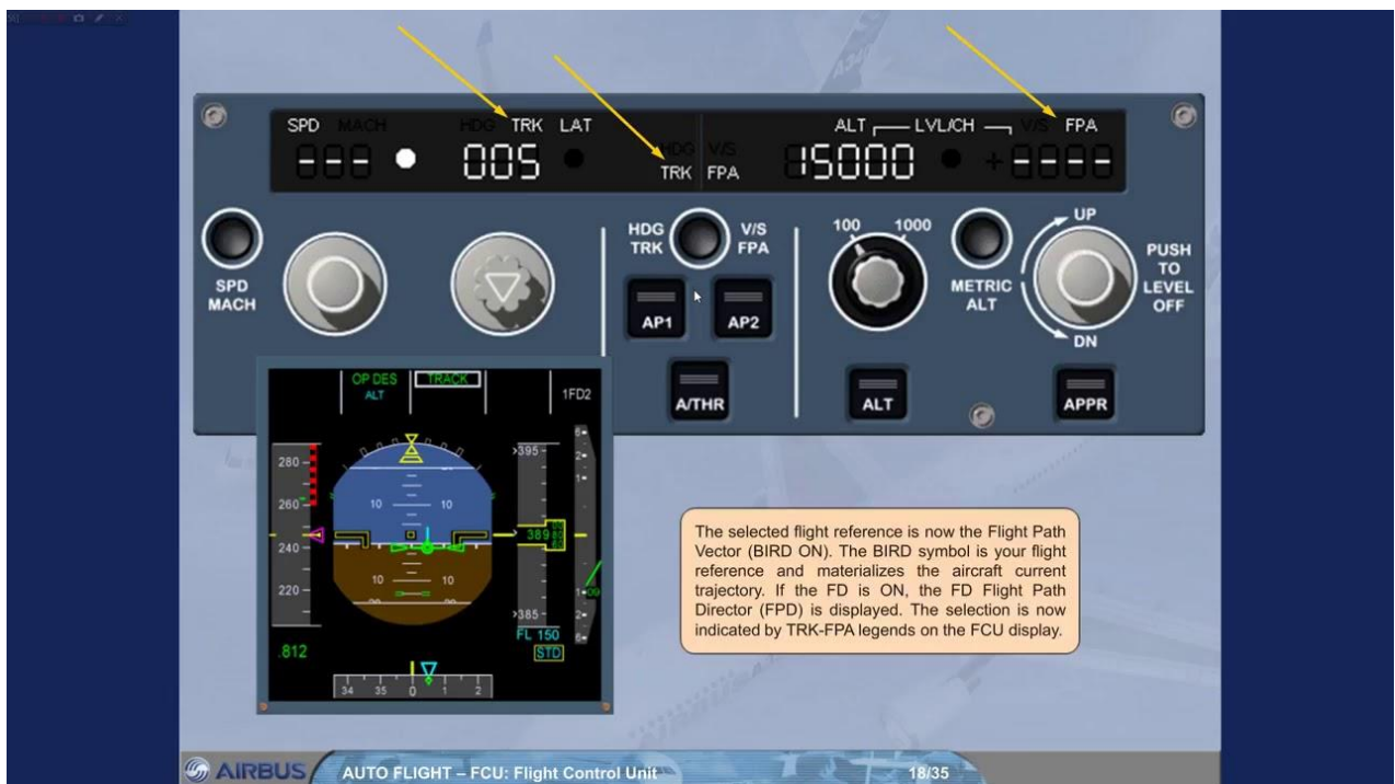
Figure 1.3. A modern flight control unit from an Airbus A340.
