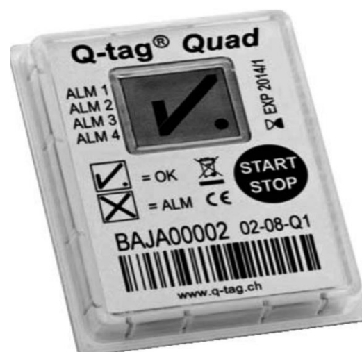
Figure 3.2 – An example of a freeze indicator
