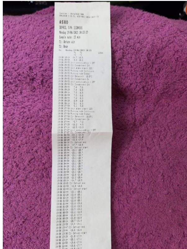
Figure 1.6 - An example of a printed temperature report from transportation
