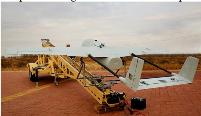
Fig. 2.6. Catapult launch UAV
