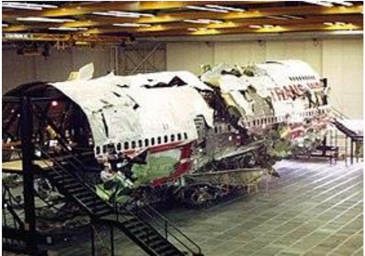
Fig. 3.4. Layout of the wreckage of Flight 800
