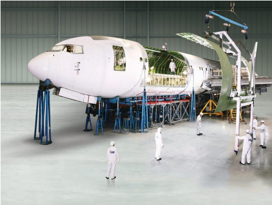
Fig. 3.1. The installation process of fuselage section with cargo door cutout on Boeing 767-300ER [20].
