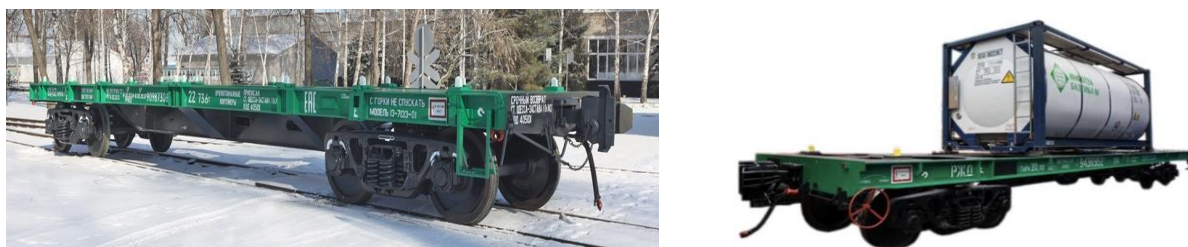
Figure 3.3 – Platform for transportation of tanks by rail transport [39]
