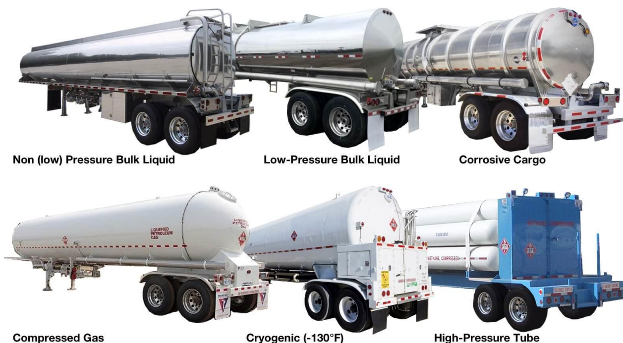
Figure 1.4 – Classification of road tankers for transportation of fuel and lubricants
