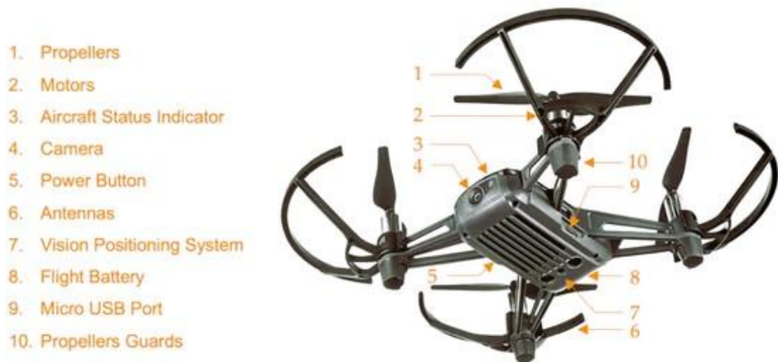
Fig.1.5.1. Basic components of Tello quadcopter
