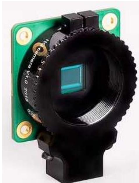
Fig. 1.10 Pi High Quality Camera without a lens
