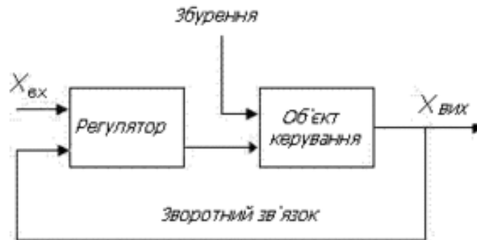
Fig. 1.5 Functional diagram of SAC with deviation control
