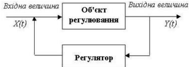
Fig. 1.2 Functional scheme of ACS
